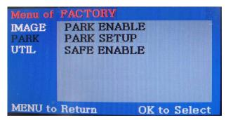
① Register the value needed on the "PARK ENABLE" as "ON" in the PARK section as shown left. (**default – ON**)
